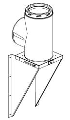
FIGURE 14 - Assembled Wall Support with Tee Cap Secured in Place
