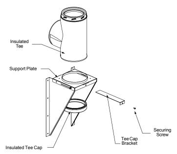
FIGURE 13 - Explosion View - Wall Support, Insulated Tee and Tee Cap, Tee Cap Bracket and securing Screw.
