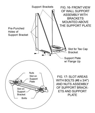
adjustability is limited to 5" from the wall (see Table 2). Install the Insulated Tee Cap as per step 15.
