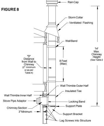
See Table 2 for maximum Chimney Heights based on Chimney Diameter and Distance from Wall The following steps will assist you in the installation of the Wall Thimble and of the Wall Support. Figure 8 shows a typical Wall Support installation through a combustible wall.
