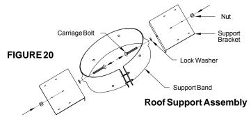
and support bracket to provide proper spacing as shown in Figure 20.
