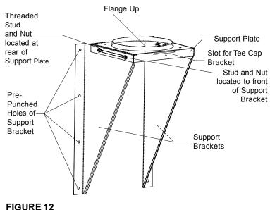
FIGURE 12 FRONT VIEW OF WALL SUPPORT ASSEMBLY
